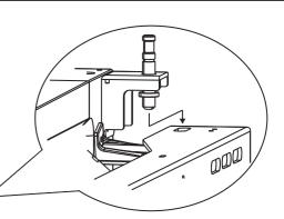
The adjuster pin is inserted through the hole of the wall brackets (top), and the monitor brackets (bottom) are inserted in the pin of the wall brackets (bottom).
