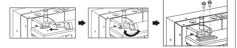
Attach stoppers. The stopper is attached with two screws each. Install the two stoppers in each monitor. You can adjust vertical position of monitor even after installing the stopper.
