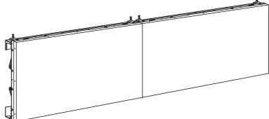
Additional monitors are set up using the same steps. Caution: When sliding the monitors to adjust spacing, DO NOT contact sides of monitors with force.
