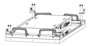
To avoid damaging the screen face, place a protective sheet on the table underneath the LCD. Make sure there is nothing on the table that can damage the monitor. Lay the monitor on the table with the screen facing down. Attach four (4) monitor brackets (top) / (bottom) to the corners of monitor with attached screws.
