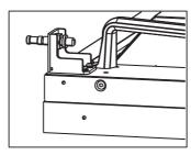
Place the adjuster pin screws in the top monitor brackets (2). Turn by hand until the adjuster pin reaches the end and stops.
