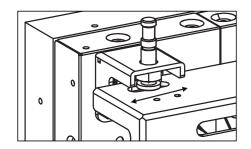
Adjustment of horizontal direction: Slide the monitor horizontally.
