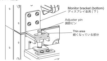
When the hole of monitor bracket attach the part where adjuster pin is thin, the monitor surface does not align. Adjuster pin must be placed correct position as shown in Step #5.
