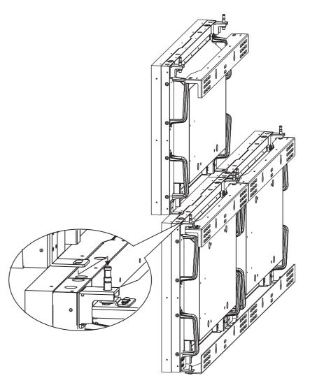
After all monitors in the the lower row are set up, begin monitor installation in the upper row. The monitor bracket (top) / (bottom) and the adjuster pin are installed just as they are on the lower monitors. The adjuster pins on the upper row monitor are inserted through the hole of the wall brackets (top), and the monitor brackets (bottom) are inserted in the adjuster pins on the the lower monitor.
