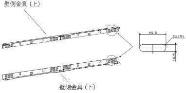
Attach wall brackets to the wall per the Installation Drawing. NOTE: Wall bracket holes are oval as shown. Please select suitable screws for attaching.
