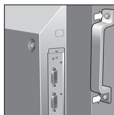
Secure the handle by 2 screws (Screw-A).
