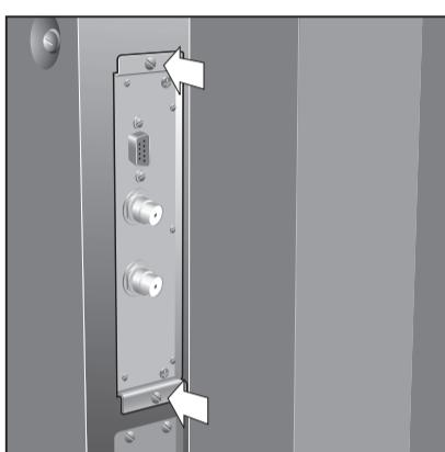
Secure SD/HD-SDI module to the monitor with 2 screws (Screw-B).
