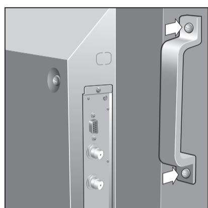
Secure the handle by 2 screws (Screw-A).
