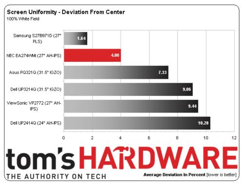
This is the second-best result we've recorded to date. The biggest deviation is at the top-center, where we measure 5 cd/m $^2$  brighter than the center. That's phenomenal performance for any LCD panel of any type.
