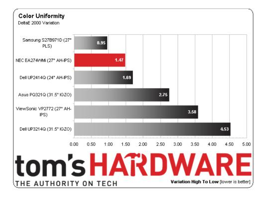
We saw no color uniformity problems with our press sample, and an error range of 1.47 Delta E backs that up. The highest value is 2.00 and the lowest is .53. All of our measurements are well below the threshold of visibility. We're using an 80-percent white field pattern, though patterns at other brightness levels look just as neutral across the screen.
