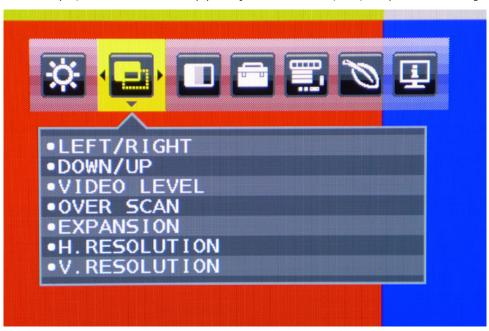
Newer monitors are doing without old-school VGA inputs. But NEC still includes them. If the image needs to be centered or expanded to fill the screen, you can do that here.
