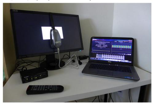
AccuPel pattern generator (bottom-left) is controlled via USB by CalMAN, which is running on the Dell XPS laptop on the right.
