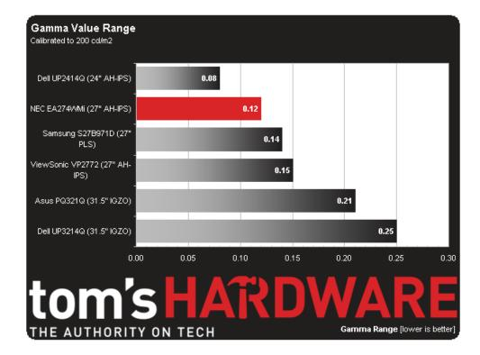
A .12 variation represents extremely flat gamma tracking. That kind of consistency is important no matter what the image source. Only three other screens of our last 22 have scored higher in this test. The tracking runs from a low of 2.09 to a high of 2.21.
