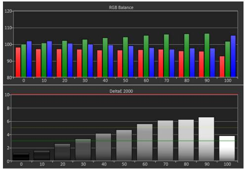
NEC EA274WMi Pre-Calibration Grayscale Tracking - Standard Mode, Color Temp 3
