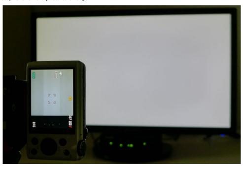
The brighter section of the camera's screen is what actually appears in the video. You can see the lights of the pattern generator in the bottom of the viewfinder. We flash the pattern on and off five times and average the results.
