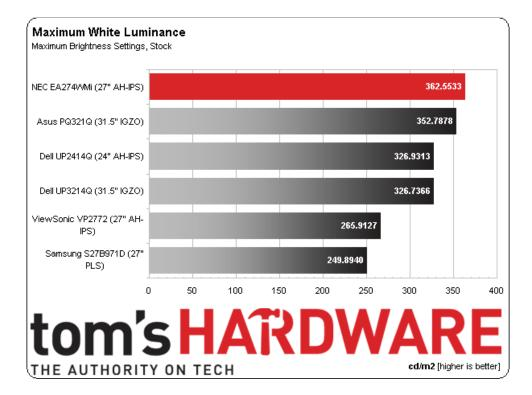
The max brightness result is measured in the EA274WMi's Standard picture mode using the Native color temp preset. Contrast is set halfway through its range (50 out of 100). You can get a little more light by upping the slider, but clipping starts at 51. The result is a little higher than the panel's rating of 350  $cd/m^2$ .
