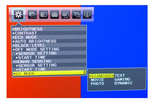
We measured all of the modes and found Standard to offer the most accurate basis for calibration. The other modes make subtle changes to gamma and color that fall outside our accepted standards. Text for instance, adds a little edge enhancement to make fonts more crisp. And Movie bumps up only the lower brightness levels. In Dynamic mode, the contrast shifts depending on image content. Take care with this setting; it can sometimes crush highlight and shadow detail.
