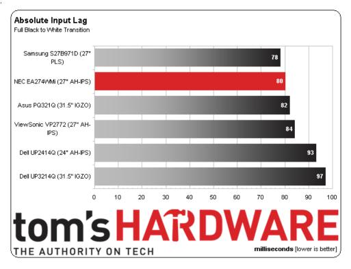
The EA274WMi is a tad quicker than other recently-tested monitors. While none of the group is classified as gaming-oriented, an input lag of 80 milliseconds is sufficient for all but the fastest titles.
