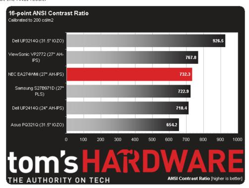
The ANSI value is a little lower than the on/off one, just like every other display that's been in our lab. Obviously this is an extreme test. As mentioned, though, it's also more real-world. Intra-image contrast is what we see in a typical image. In the case of the EA274WMi, the drop is less than nine percent. I consider that to be excellent.
