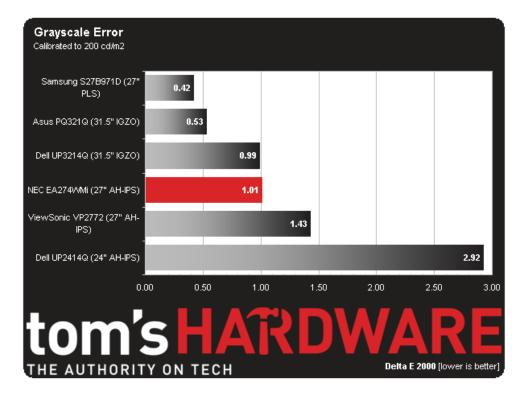
A 1.01 Delta E error is pretty close to the best displays we've tested. As you'll see later in the color gamut tests, calibration improves accuracy across the board.
