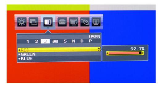
Presets 1, 2, 3, and 5 are adjustable, and they start at color temps of 9300, 8200, 7500, and 5000 Kelvins, respectively. Number 3 is closest to the preferred 6500 K setting. sRGB, N (Native), and D (DICOM) (used in medical imaging) cannot be changed. P is for Programmable and works with a PC app to control the EA274WMi, but it only addresses gamma, which is fine as-is.
