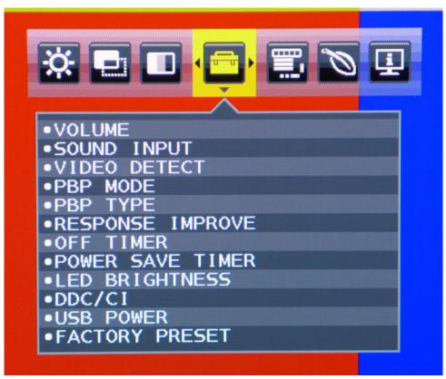
Volume controls both the internal speakers and the headphone output. Since audio signals can come in via a 3.5mm jack, HDMI, or DisplayPort, Sound Input lets you select the source.
