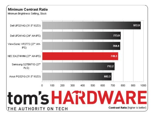
The minimum contrast ratio drops around 22 percent from the max number, yielding a decent result (even if it's less consistent than the last few monitors we tested). The other five in this group all measured closely in their maximum and minimum contrast tests. Hopefully, the calibrated result will be somewhere in between.
