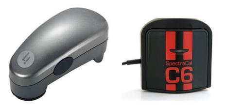
The i1Pro is very accurate and consistent measuring color on all types of displays, regardless of the backlight technology used. When we just need a luminance value, the C6 works better, especially in low light.
