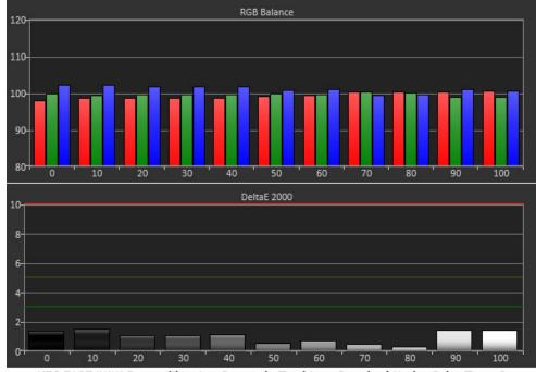
NEC EA274WMi Post-calibration Grayscale Tracking - Standard Mode, Color Temp 3
