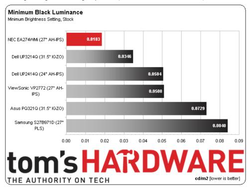
Our measured minimum black level trounces the other monitors in the group, but that is mainly because of the extremely dim backlight. At  $50 \text{ cd/m}^2$  max, the black level would put NEC in fifth place, which is an otherwise typical performance for a 27-inch QHD screen based on an LED-lit IPS panel.
