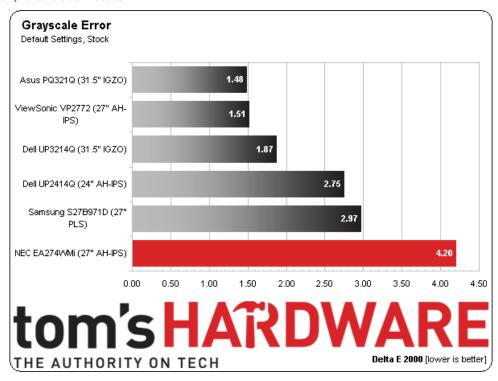
For a pro-level display, this is below-average performance. Many of the screens we test now fall below the three Delta E threshold without calibration. Our result of 4.20 Delta E represents the Color Temp 3 preset. Native is slightly higher at 4.38, and sRGB is the highest at 4.77.
