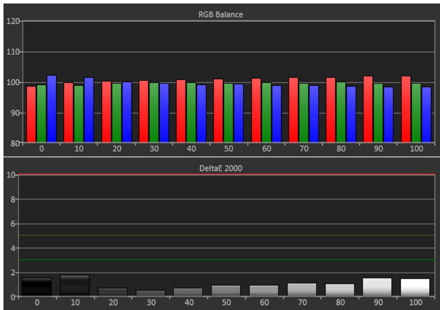
NEC PA322UHD Grayscale Tracking - sRGB Mode, Pre-calibration
