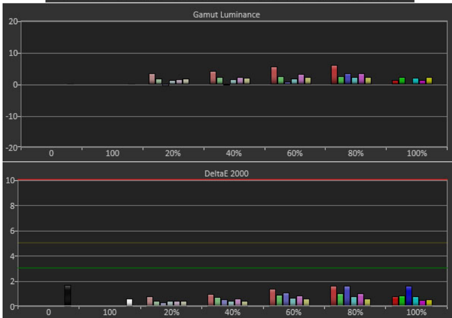
NEC PA322UHD Chromaticity - sRGB Mode Calibrated
