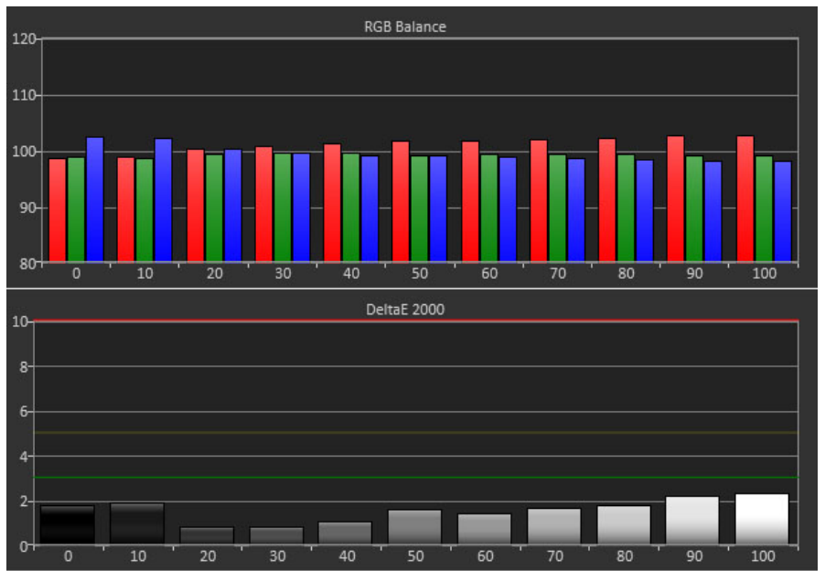
NEC PA322UHD Grayscale Tracking - Adobe Mode, Pre-calibration
